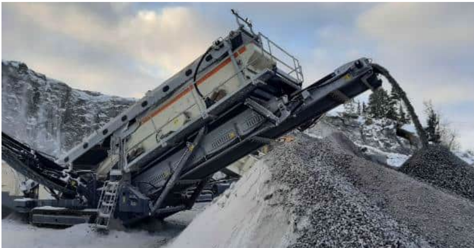
Type H12-8 robust product conveyor with 4300 mm discharge height and belt speed of 1,85 m/s enables high stock pile capacity .
