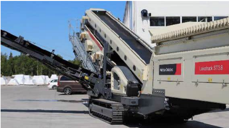
Belt conveyor for lifting the material from feeder to the screen . Conveyor is equipped with spreader plate distributing even material flow on the screen.
