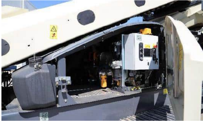
Power unit is designed for easy maintenance .
