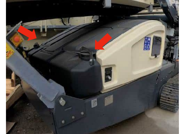
Integrated fuel tank enables re-fueling from both sides
