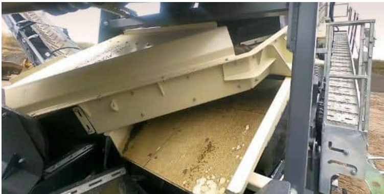
Diverter chute with removable wear plates to mix products. Horizontal load zone minimizes spillage .
