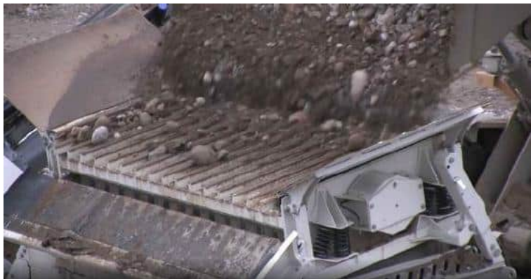
Feeder module can be equipped with tipping grid , two deck vibrating grid or rock box depending feed material and the feeding arrangement in the application.
