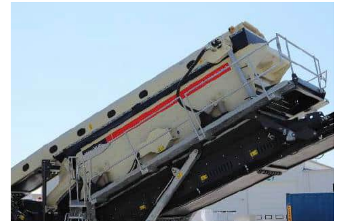
Large platforms for easy and safe access to all service locations.
