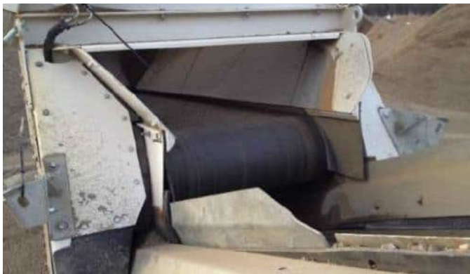
Powerful belt feeder with well designed feed box and adjustable belt speed ensures seamless flow .
