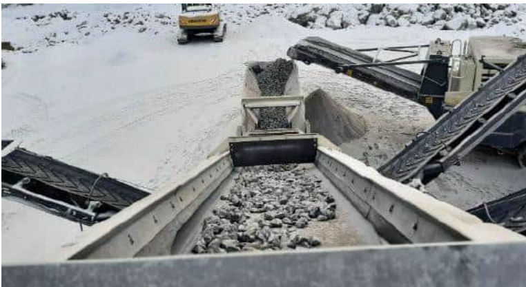
Lifting conveyor with 1050 mm width and adjustable maximum speed of 1,8 m/s enables high capacity .
