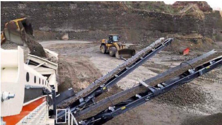
Adjustable angle for reduced rollback and easier closed circuit .
