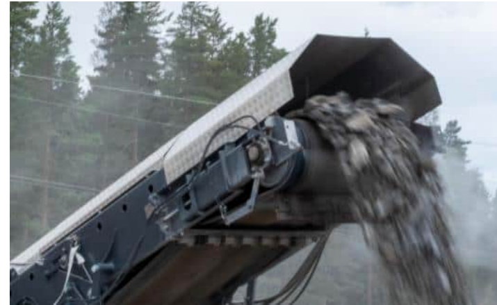
Dust encapsulation includes aluminum sheet covers of conveyors for improved dust control.
