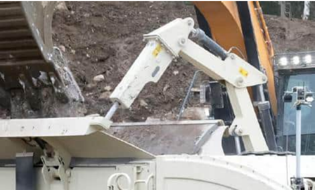
The hydraulic hammer can be installed to the Lokotrack to break the oversize material in the crusher cavity. It is a safe and quick way to clear and prevent blockages during crushing.
