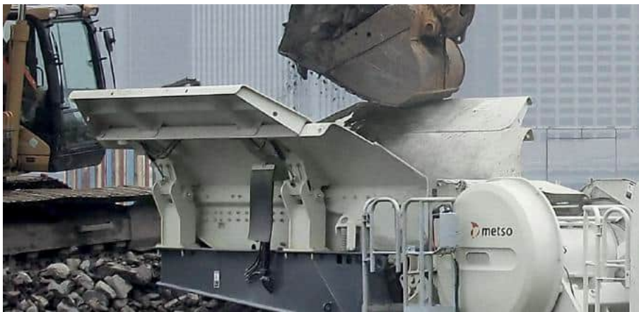
Option available for hopper extensions (9 m 3 ) to add more capacity.
