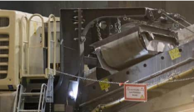
Overband magnetic separator on main conveyor having stainless steel discharge chutes. Separates ferrous objects from the crushed material and transfers those to a separate pile beside the machine.
