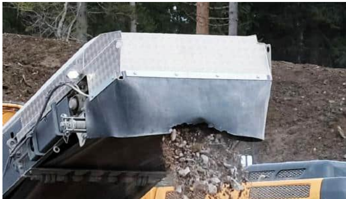
Aluminum discharge hood with hanging rubber for conveyors. Discharge hood reduces dust from the conveyor discharge point.
