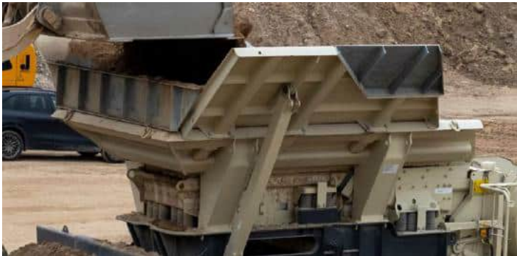
Feed hopper extensions to add more capacity and enable wheel loader feed.
