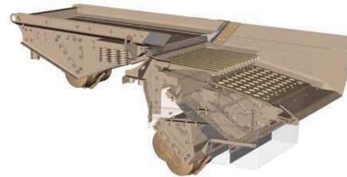
Alternative vibrating feeder with scalper and feeder. Two vibrating units with specific movement provide optimized separation of sticky material.
