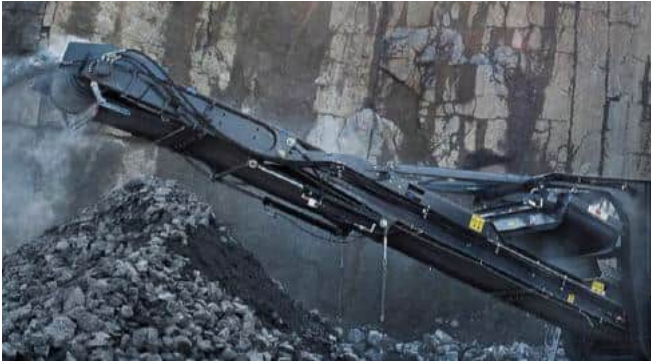
Extended main conveyor enables increased stockpile capacity and easy adaptability to Lokotrack combinations.
